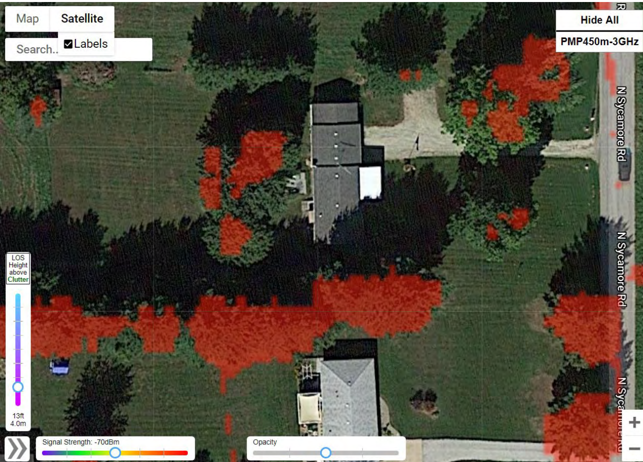
LOS Coverage at 13' is non-existent
