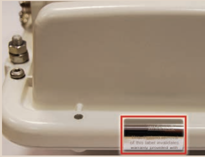
3. Anti-tamper labels are strategically located on a PTP 600 ODU with connectors.
