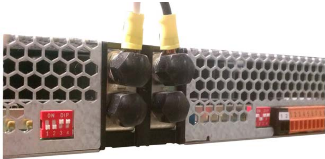
Figure 33 56 VDC power supply DC connection
