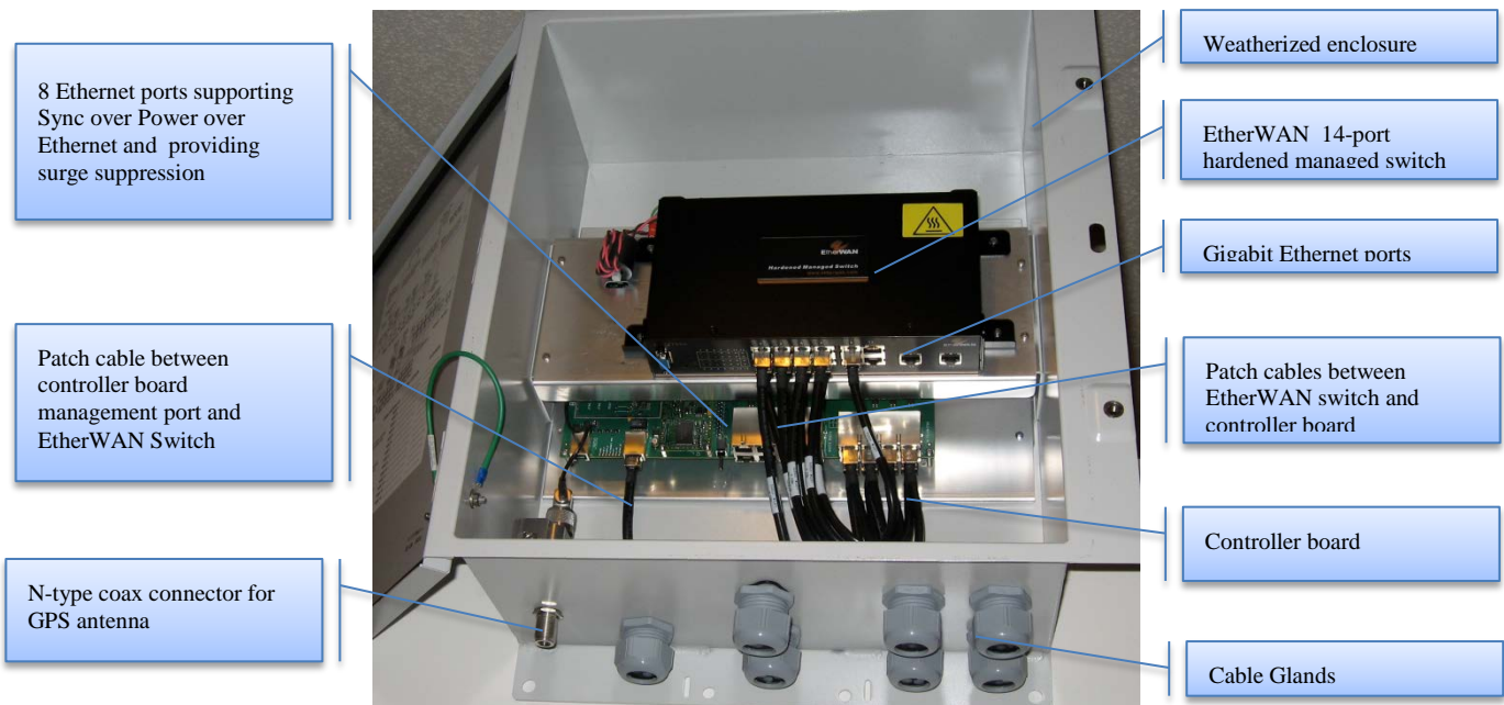
Figure 3 CMM4 internal view, including cable glands
