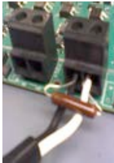
Figure 36 Resistor when using both 56 VDC and 30 VDC power
