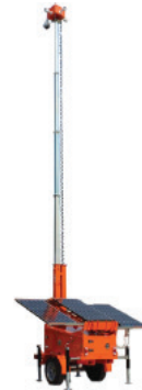
3. Trailer-mounted mast that can be pulled behind a vehicle incorporating solar panels and battery
