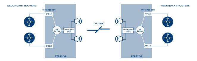
In this network configuration, a pair of redundant MPLS routers are connected to a PTP820G Chassis at each end. The PTP820G is configured with 1+1 Hot Standby for radio redundancy. The implementation needs to make sure that on a sunny day, all four routers can talk to each other. Failure of any of the 1+1 radios will not affect the traffic going through the routers if the 1+1 radio link is up.
