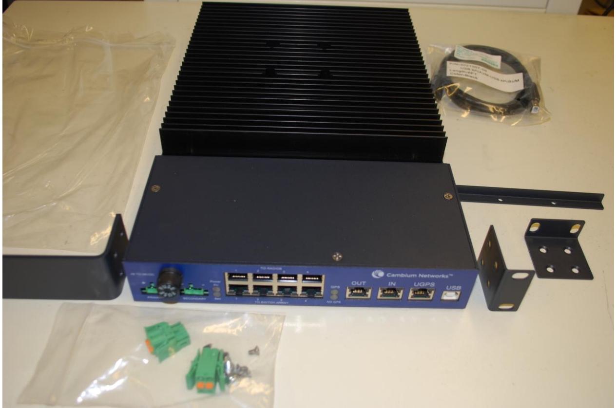
Figure 19 Installing a Single Injector
