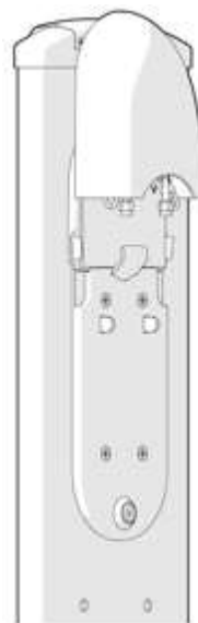
Figure 17 Connectorized radio sector antenna
