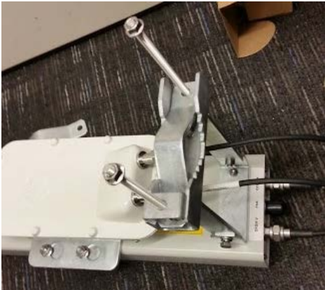
Figure 94 Lower bracket attached to AP antenna
