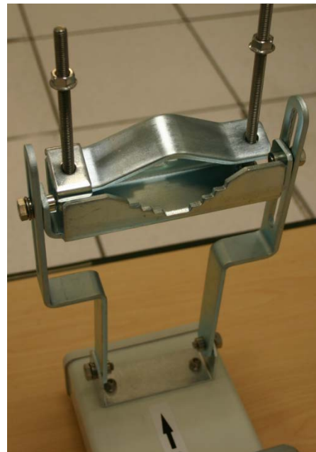
Figure 100 Assembled upper bracket connected to AP antenna
