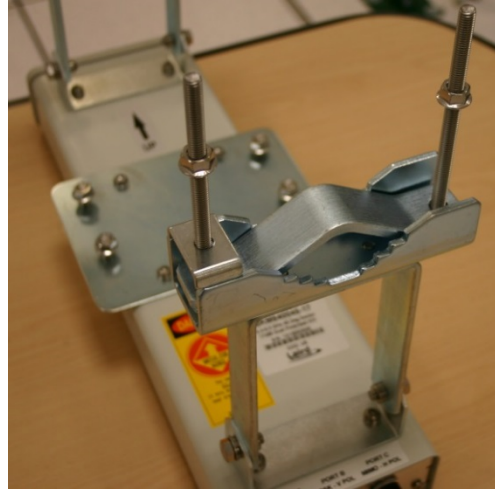
Figure 103 Attaching bracket to the rear of the AP
