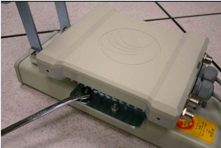
Figure 104 Lower bracket attached to AP antenna
