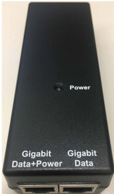
Figure 19 -20 to 32 VDC Power Injector interfaces
