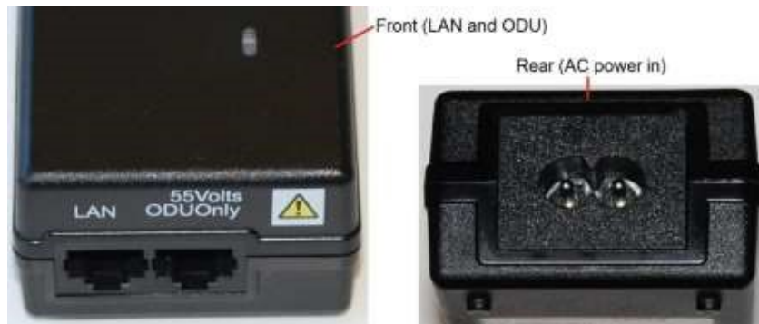
Figure 9 AC Power Injector interfaces
