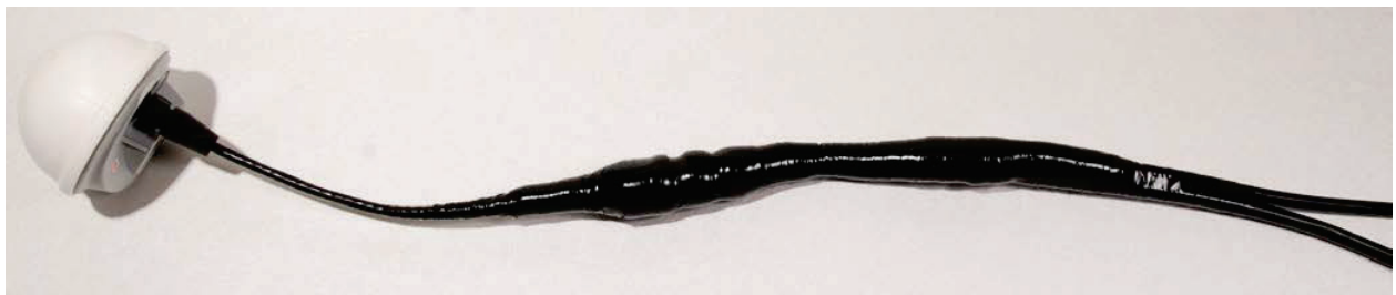
Figure 114 Grounding and weatherproofing example for GPS adapter cable
