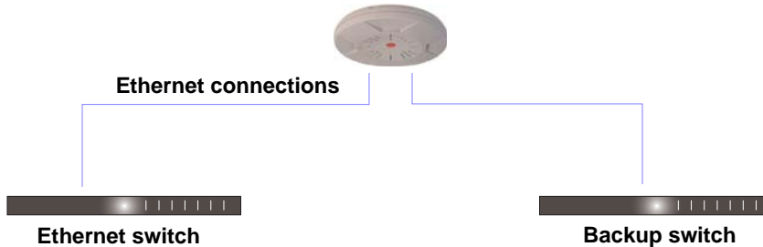
Figure 24. Switch Failover Protection
