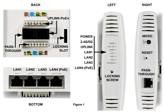
The wall AP has the following ports and jacks. For the UPLINK-PoE+ and Pass-Through ports, you may use either an RJ-45 or a punch-down connection.
