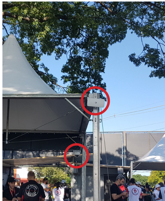
Dahua cameras (bottom) were connected to the cnVision Client MINIs (top) which provided mid-range coverage.
