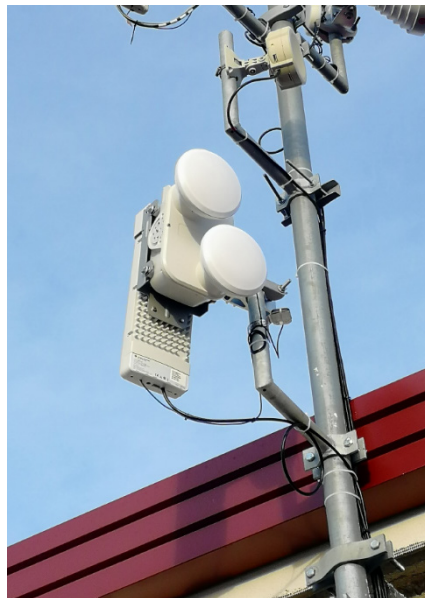
Small form factor dual horn antenna uses less tower space
