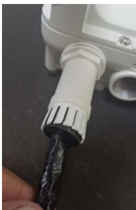
Figure 124: Fitting the gland body
