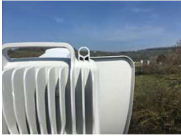
Figure 81: Locking the fine elevation adjuster
