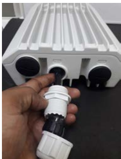
Figure 98: Removing the latch of the RJ45 plug
