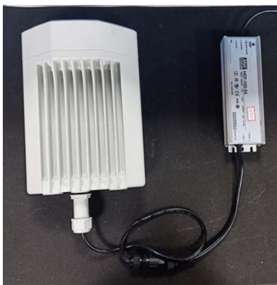
Figure 103: Connecting the output side of AC/DC PSU
