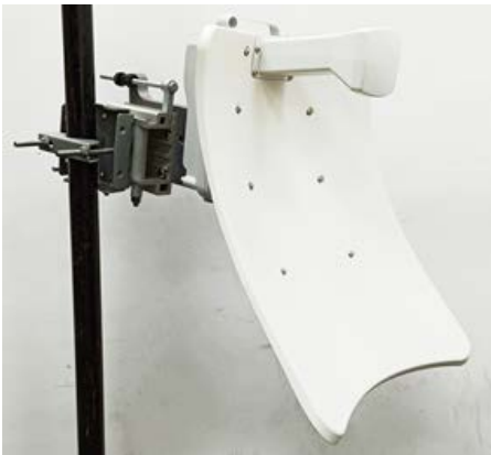
Figure 76: Locking the antenna alignment
