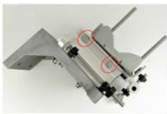
Figure 71: MB Screws located in the slots in the bracket body
