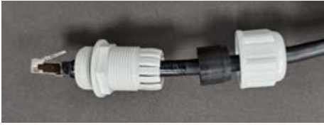
Figure 93: Fixing the gland nut
