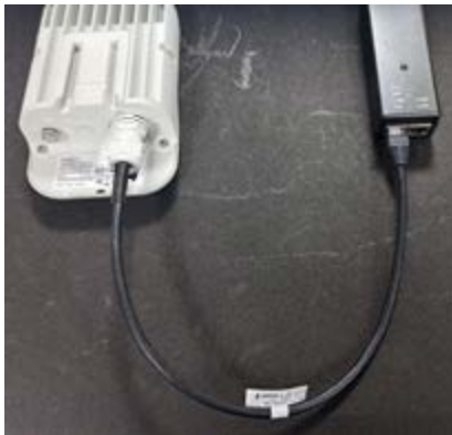
Figure 113: Connecting the V1000 power injector
