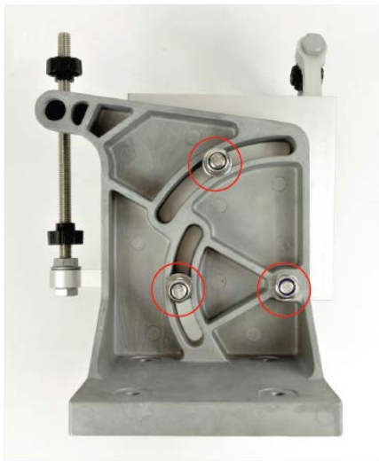
Figure 70: Plain washers and M8 Nyloc nuts on the back of the bracket
