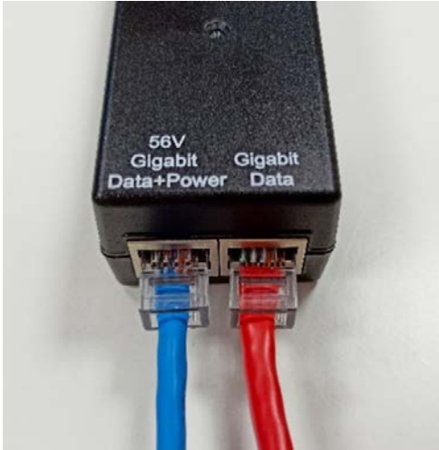
Figure 113: Connecting the V1000 power injector
