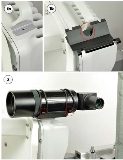
Figure 82: Attaching the telescope
