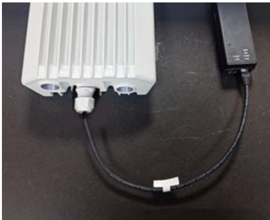
Figure 105: Connecting the power injector to ODU drop cable
