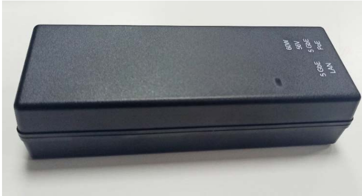
Figure 29: PoE power supply to V3000 or V5000
