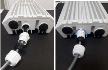
Figure 94: Connecting the RJ45 plug
