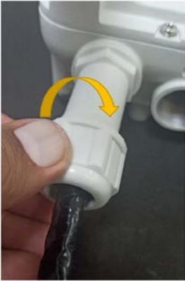
Figure 125: Fitting the gland nut
