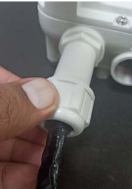
Figure 126: Fitting the gland nut to the rubber seal
