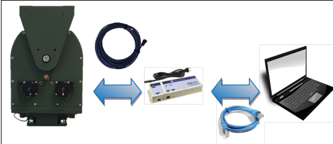
Figure 1: Step 1 - Setup of TD-90 to pre-configure
