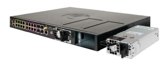
Ensure that the CRPS is installed in the correct orientation. The handle will be located on the left, while the latching tab will be located on the right side of the CRPS.
