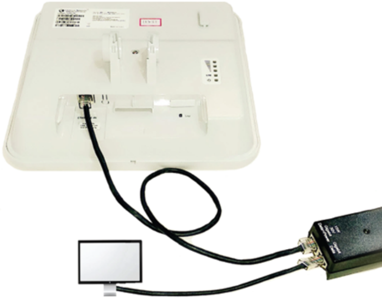
Figure 1: Installation of Tyndall 101 to PoE adapter
