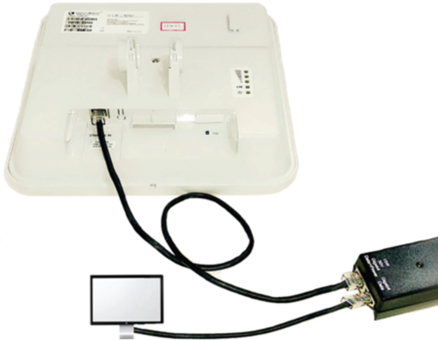
Figure 28: Installation of Tyndall 101 to PoE adapter
